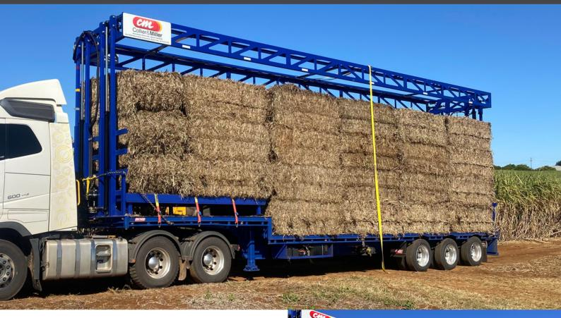
The Collier & Miller Hay Cartage Trailer Frame converts your drop deck semi into a high-capacity hay transporter, carrying up to 42 large rectangular bales within NHVR regulations.
